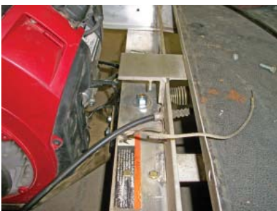
Connect engine ground cable to valve cover mounting bolt.
